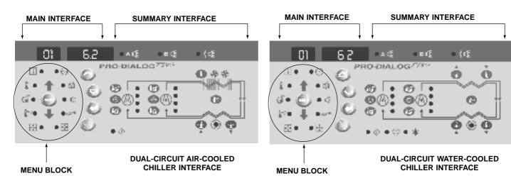
The local interface enables a number of operating parameters to be displayed and modified.
